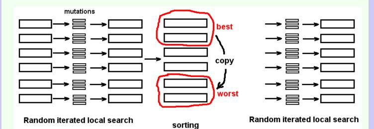
Mutations and evaluation of obtained solutions are done in parallel on a Graphics Processing Unit (GPU)
